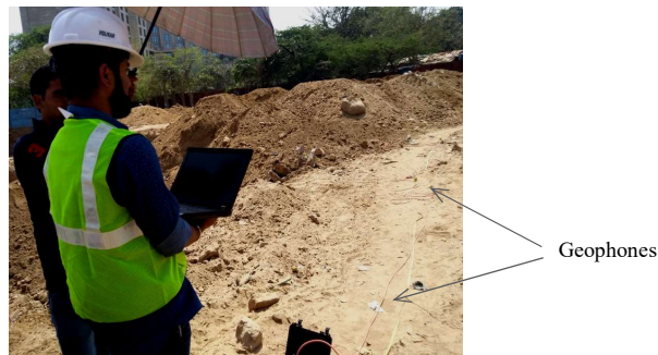
Fig. 4. Seismic Refraction Test – Data Acquisition in progress.
